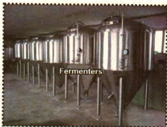
Figure 17.5: Fermenters used in food and pharmaceutical industry
