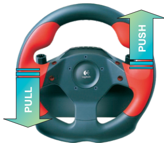
Figure 4.24: It is easy to turn a steering wheel by applying a couple.
